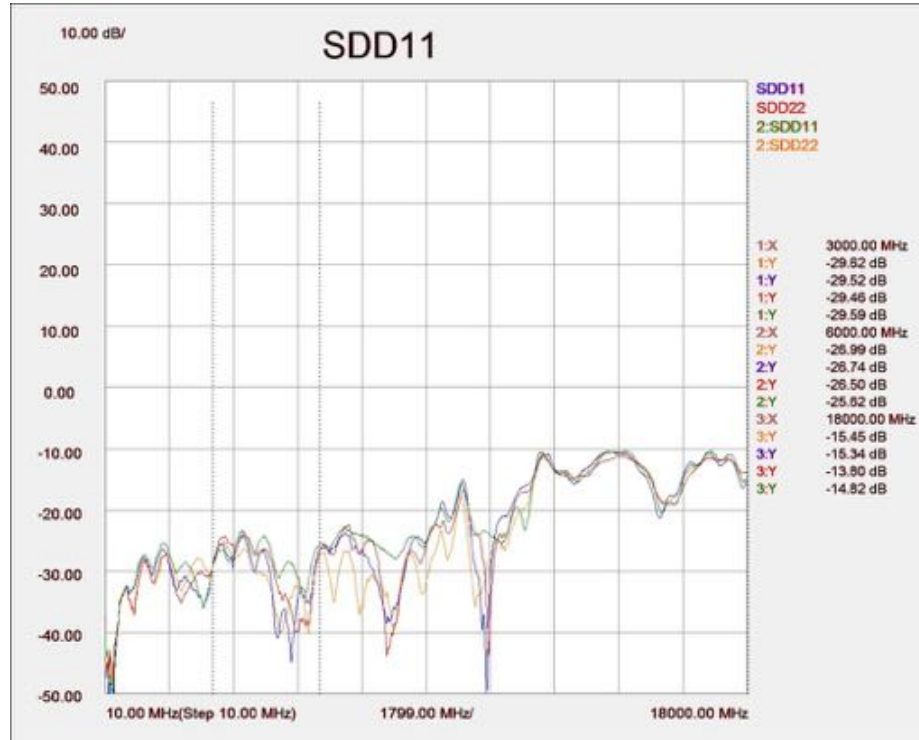
Figure 19. Typical plug TPA balanced return loss, differential termination replacing Mini-SAS HD connector
