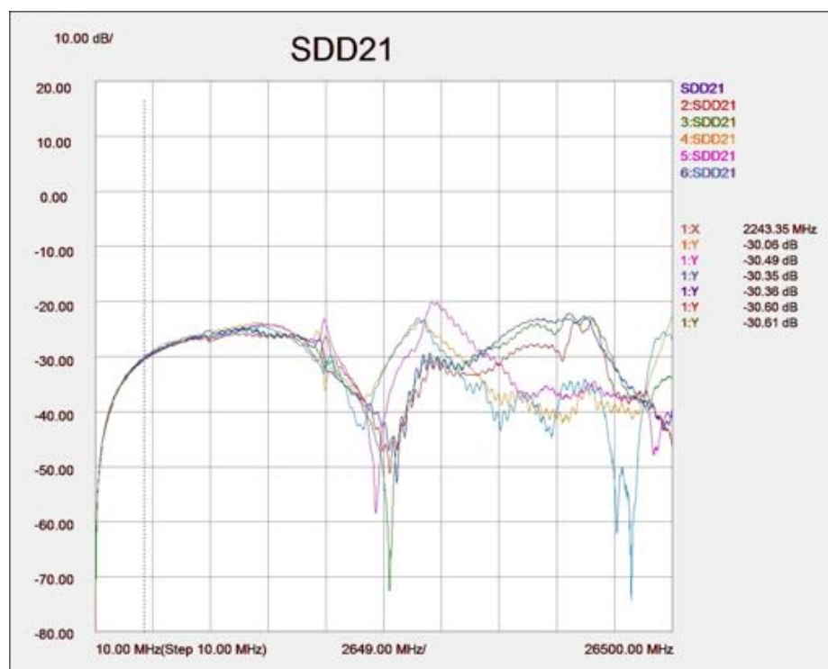
Figure 13. Typical Differential NEXT of TMDS, without connector (top) and with mated connectors (bottom), adjacent lanes, all lanes terminated at both ends
