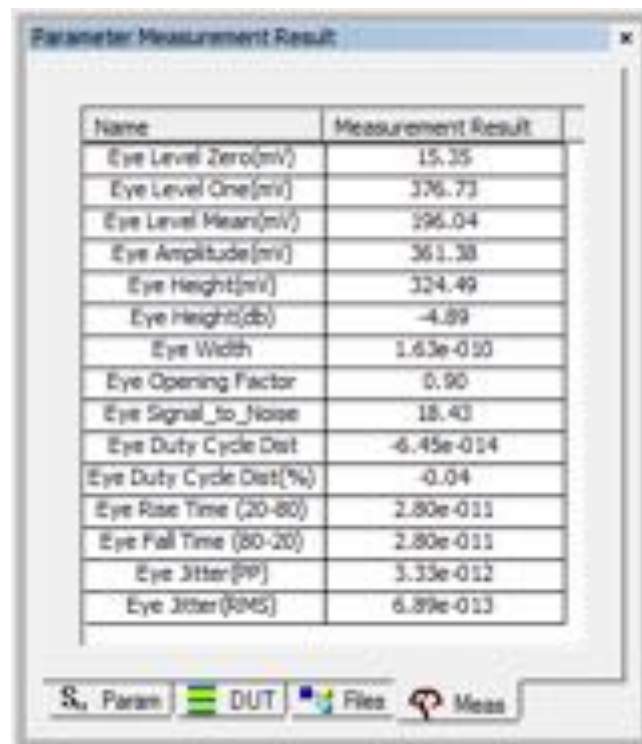
Figure 7. Typical TMD5 mated pair 6 Gb/s eye measurements, without de-embedding
