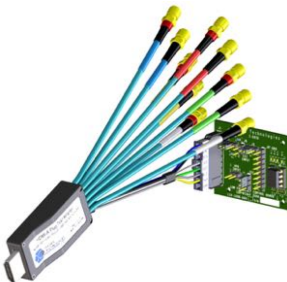
Figure 4. HDMI2-TPA-E (E-EDID/Low Frequency Control Board) mated to a HDMI2-TPA-P (Plug) Test Adapter
