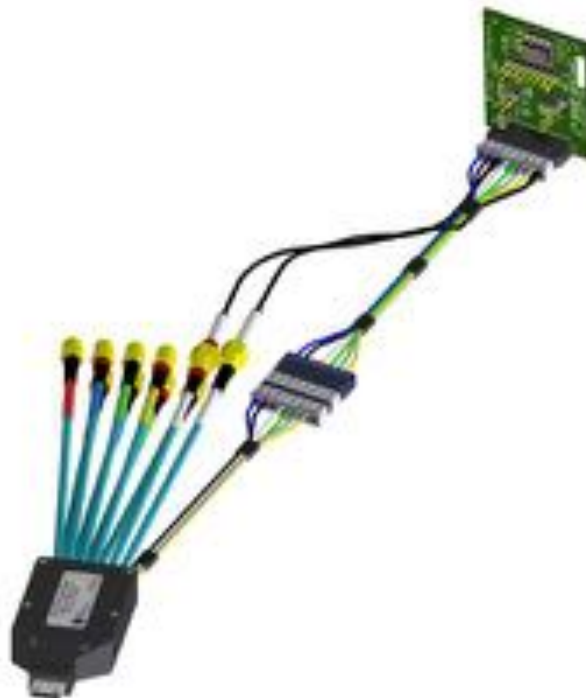
Figure A-4. E-EDID/Low Frequency Control Board utilizing the HEAC adapter cable assembly between the HDMIC-TPA Plug and the EDID/Low Frequency Board for non-HEAC testing
