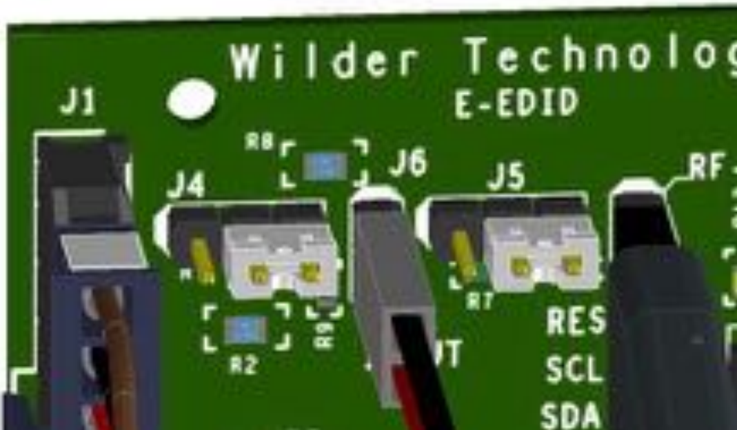
Figure A-10. Jumper positions for CEC power through the 27k Ohm resistor and 1k Ohm resistor to DDC/CEC ground on the E-EDID/Low Frequency Control Board.
