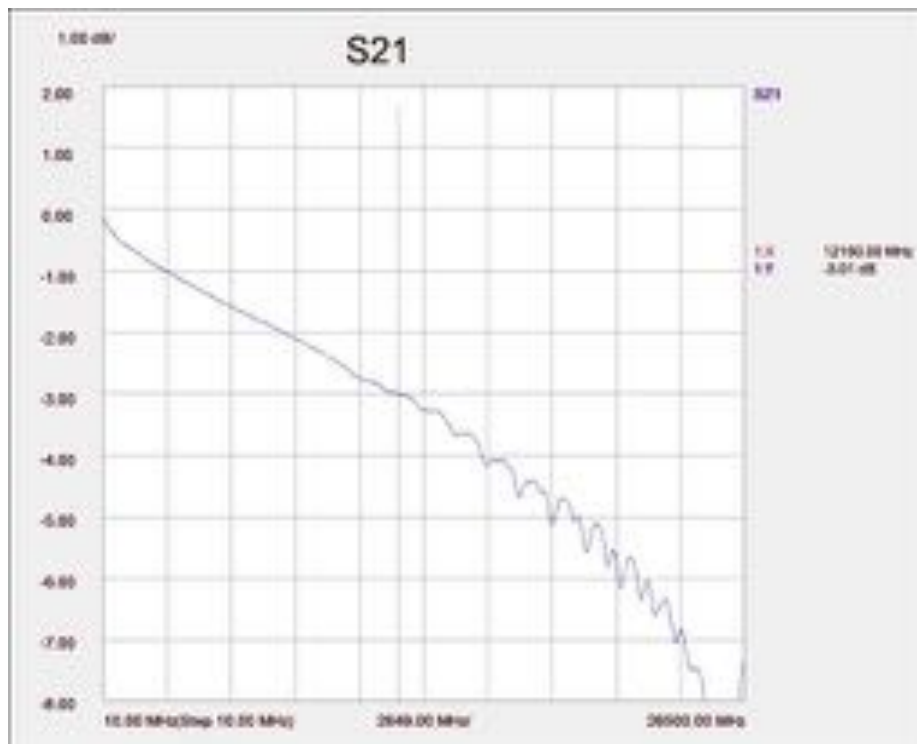
Figure 7. Typical 2X-THRU insertion loss
