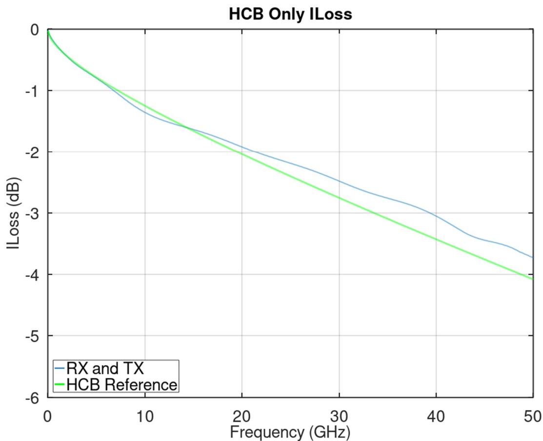
Figure 9. Plot of QSFP112 HCB Insertion Loss
