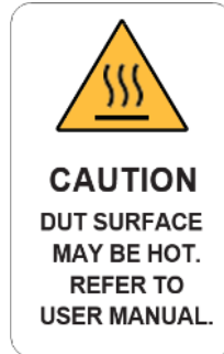
Figure 7. Caution Label, IEC 60417. Caution, Hot Surface
