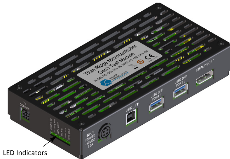
Figure 8. Titan Ridge Generation 3 Microcontroller LED Status Indicators
