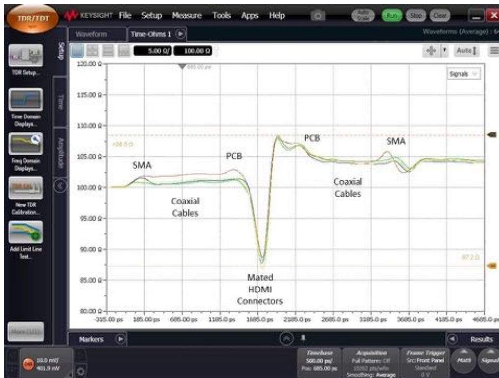
Figure 14. Typical differential TDR of TMD5, HDMI2-TPA-P connected to HDMI2-TPA-R at 100 ps Rise Time
