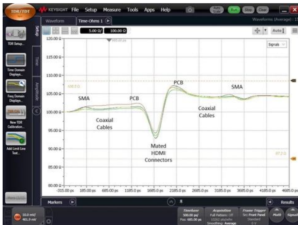
Figure 15. Typical differential TDR of TMD5, HDMI2-TPA-P connected to HDMI2-TPA-R at 200 ps Rise Time
