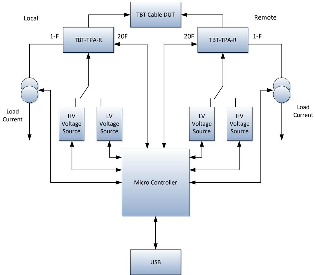
Figure 5. Thunderbolt Cable Power Controller Block Diagram
