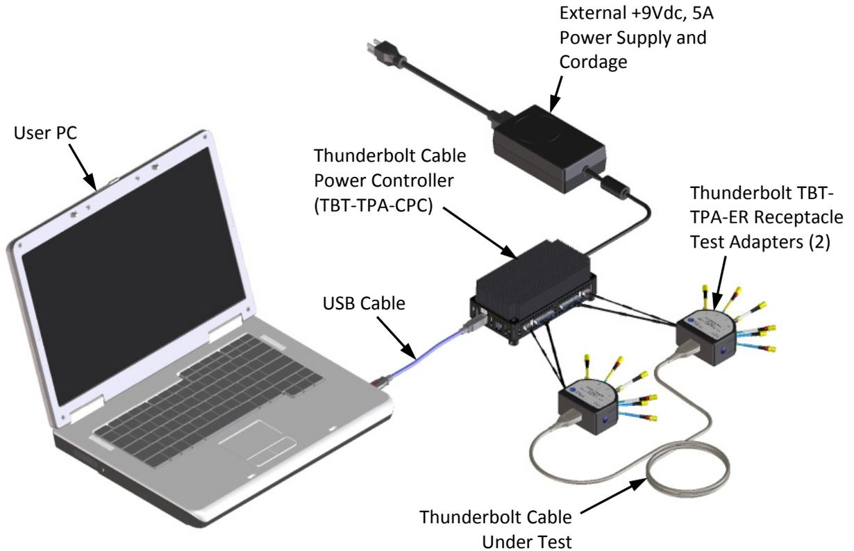
Figure 4. Two TBT-TPA-ERs (Receptacle Test Adapters) mated to a TBT-TPA-CPC (Thunderbolt Cable Power Controller)
